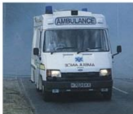
Figure 13.7 Some emergency vehicles have mirror writing on their bonnets so that drivers in front can read the name when they look in their mirrors.
